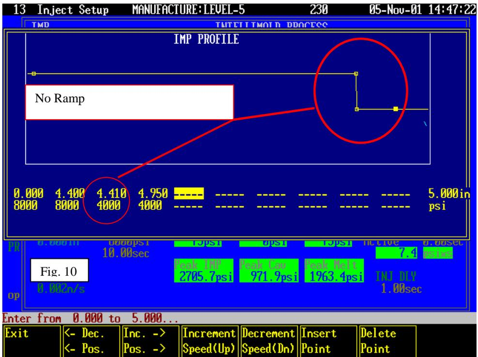
Notice the built in ramp on figure 9, to eliminate any unwanted ramps in the Van Dorn control specify the start position and pressure as well as the end position and pressure.
