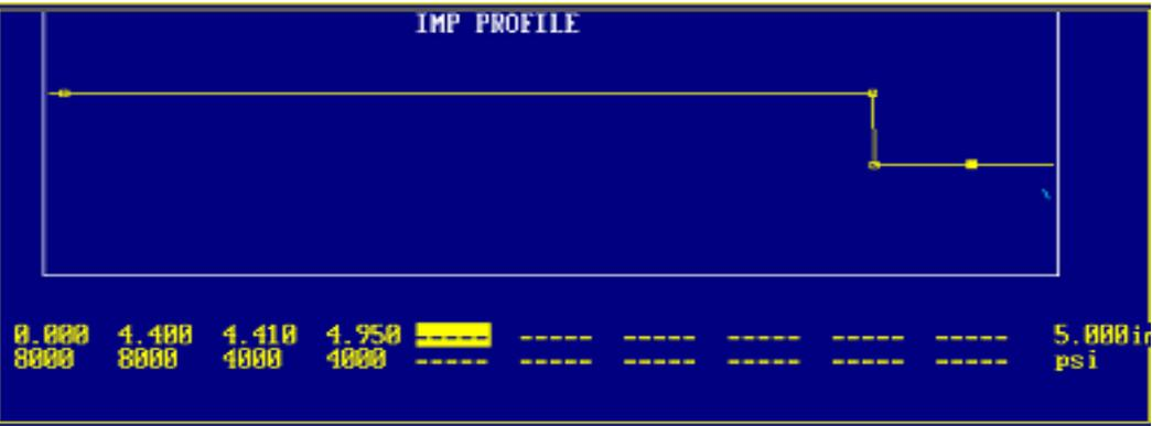
Fig. 7 (Left) Demonstrates the ability to do a four-segment profile with IMP pressure Vs Position. This profile is only active when IMP Control is on.
