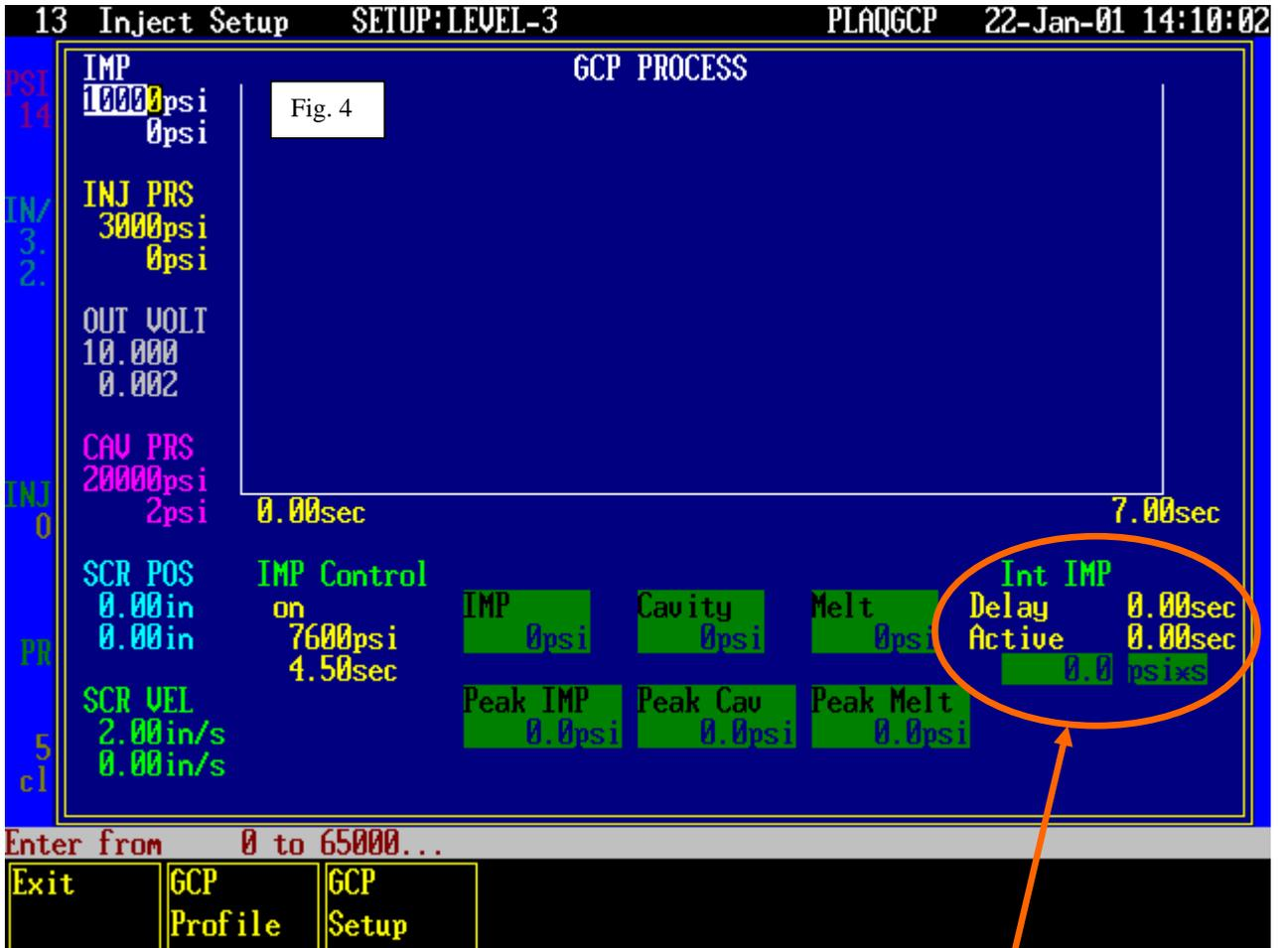
Int IMP (Integral IMP) gives the ability to calculate 1<sup>st</sup> Integral in a PSI vs. Time format. This is used to calculate Rheology. If you refer to the figure below it shows a typical IMP curve, as it would be displayed on the Main IntelliMold (GCP) Screen. By specifying a delay to start time and an active time you are able to calculate the area under the IMP line, or otherwise known as the 1<sup>st</sup> integral.
