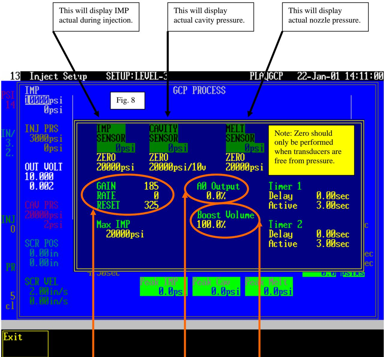
In this field you are able to adjust the GAIN, RATE, RESET. Gain = Proportional, Rate = Derivative, Reset = Integral. The tuning values you assign in this field are used on the calculated process variable. (IMP) It is only used when IntelliMold (GCP) is turned on.
