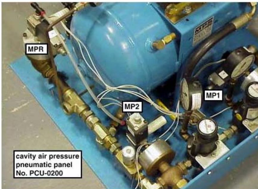
Located on the left is a picture of the most common pneumatic panel used. It clearly shows the location of MP1 (GCP1), MP2 (GCP2), and MPR (GCPR). There are however more than one option of pneumatic panels available. For more information contact your IntelliMold representative.
