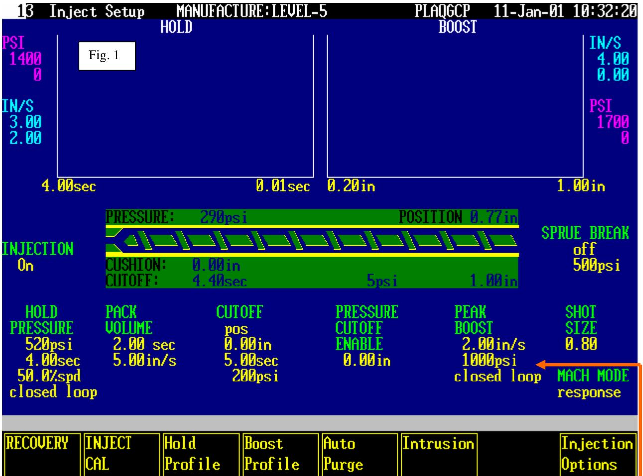
Above screen is the conventional injection screen from a Pathfinder 5000 Control. Although it may vary slightly, It is pretty common among the Pathfinder series. It is from this screen that you access the Intellimold System (GCP). Note: IntelliMold is also known as GCP on earlier systems.
